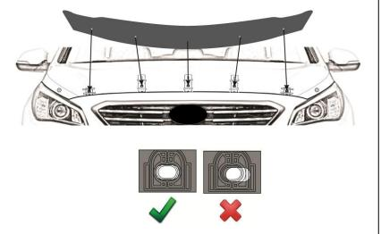
5. Dry fit the remaining pedestals using tape strips supplied or masking tape to temporarily hold them in position.
