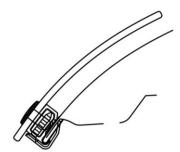
15. Peel and fold two (2) of the large anti-abrasion film pads in half over the hood edge aligned with the inner holes of the deflector in the area above the headlights.
