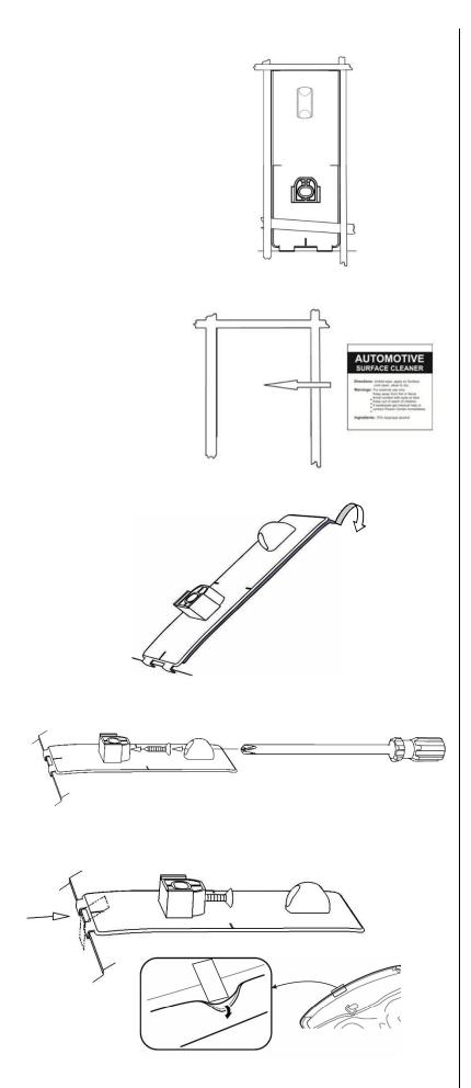
7. Remove the hood protector and outline the perimeter of the pedestals with masking tape or the re-usable tape strips supplied.
