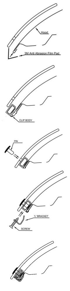
14. Peel and fold the four (4) large anti-abrasion film pads in half over the hood edge aligned with the outer holes of the deflector in the area above the headlights.
