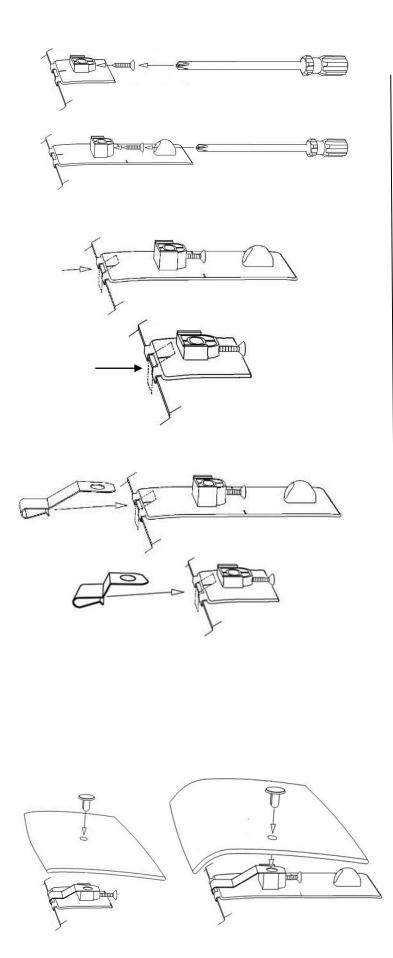
12. Start a screw into each pedestal a few turns. The tip of the screw must not protrude into the hole where the attachment pin will later install.
