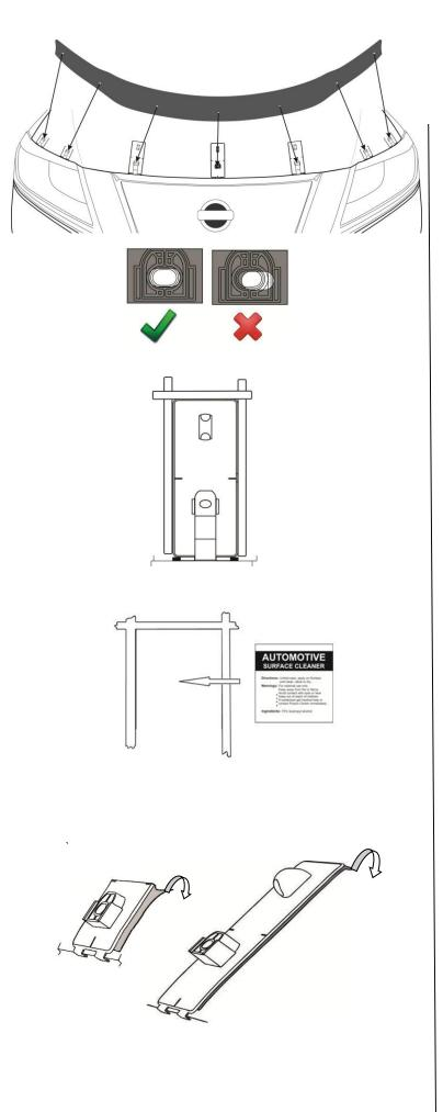
8. Place the hood protector on the pedestals to confirm proper positioning. Ensure the holes in the protector align with those in the pedestals. If necessary, reposition the pedestals so all attachment positions are correct and the protector is well centered.
