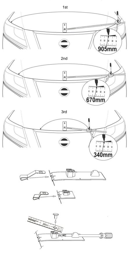
5. The positions of the pedestals are shown in the **illustrations**. Mark the hood edge with a felt pen or grease pencil at these locations.
