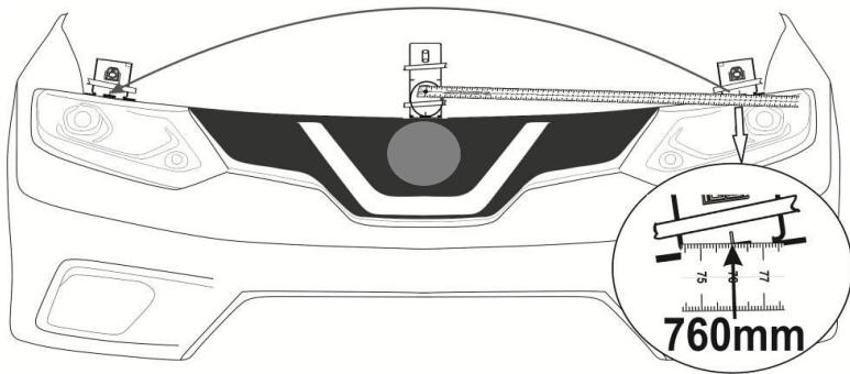
\* Tape measure is always located below the measuring point\*
