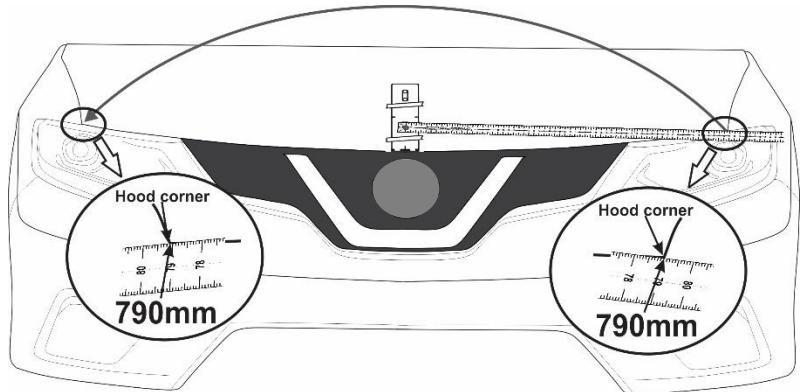
\* Tape measure is always located below the measuring point\*
