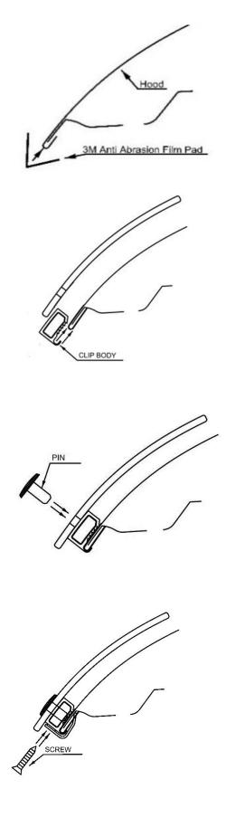
12. Peel and fold the four (4) large anti-abrasion film pads in half over the hood edge aligned with the outer holes of the protector in the area above the headlights.
