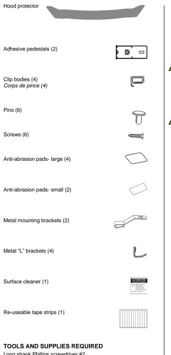
Long shank Phillips screwdriver #2 Tape measure Masking tape
