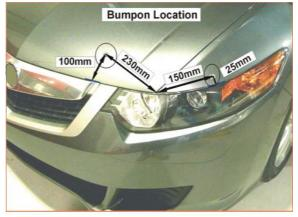
Open the hood. Peel and fold anti-abrasion film pads in half over the edge of the hood in the four (4) locations shown in the illustration below.
