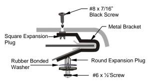
Install the remaining two (2) metal brackets (Type 1) over the hood edge, at 245mm location. See *Illustration in step 3*. Note: the #8 x 7/16" black screw and hood guard are not put in place until step 15.
