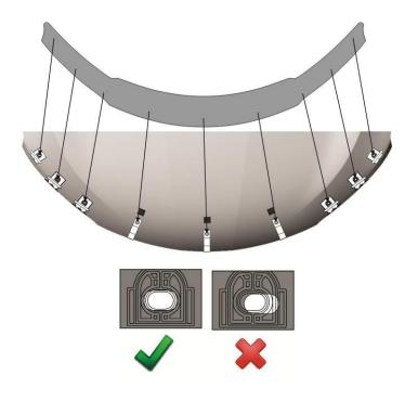
Place the protector temporarily onto the metal brackets, aligning the holes in the protector with the holes in the metal brackets. This step will allow you to check the position of the adhesive pedestals and adjust if necessary.
