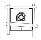
8. Remove the hood protector. Outline the perimeter of the adhesive pedestals with the tape strips or masking tape.
