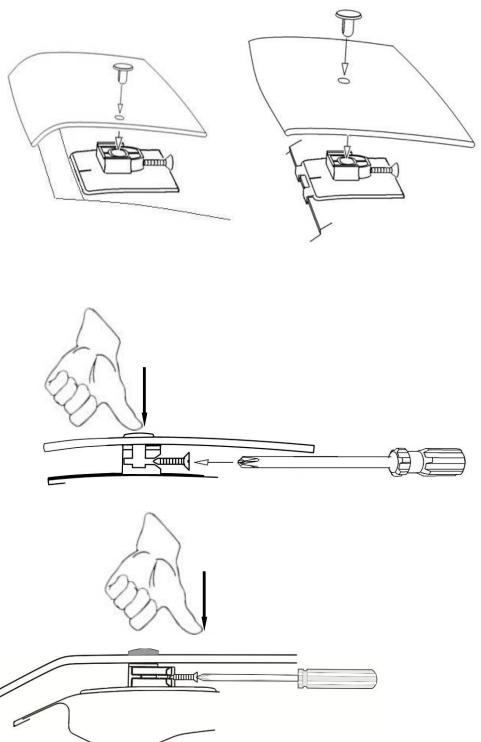
13. Starting at the inner most pedestal and working outward, insert a pin through the protector and into the pedestal. Maintain pressure on the head of the pin to ensure the protector is seated against the pedestal and tighten the screw until snug. Do not over-tighten!
