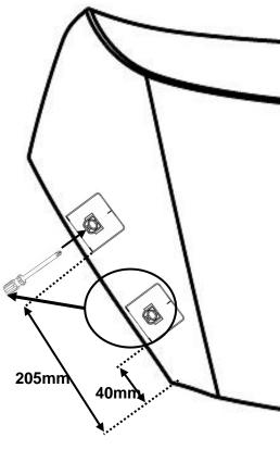
8. The positions of the pedestals are shown in illustration. Use the corner of the pedestal for the measurements. The pedestals should have an even 2mm gap from the edge of the hood to the bottom edge of the pedestal
