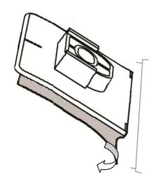
Remove the protective backing from the adhesive on the pedestals and install on the hood surface.
