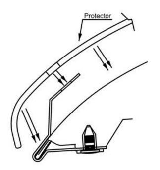
Place the protector temporarily onto the metal brackets aligning the holes in the protector with the holes in the metal brackets. This step will allow you to confirm the position of the adhesive pedestals.
