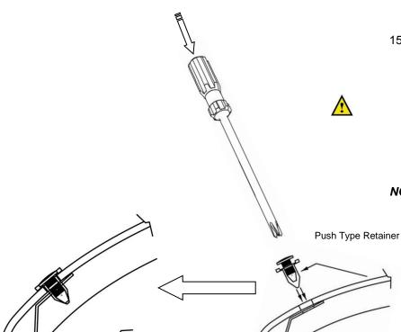
15. Place the hood protector on the hood resting on the two (2) metal brackets; align the 2 center holes in the protector with the holes in the metal brackets. Insert a "push type retainer" through the hole in the protector, and into the bracket. Ensure the protector is well seated against the surface of the metal bracket, and push the center pin of the retainer assembly to lock it into place.
