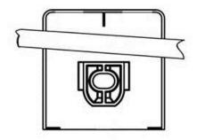
7. Dry fit the adhesive pedestals using masking tape or the repositionable tape strips supplied to hold them in position.
