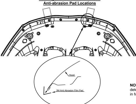
Open the hood of the vehicle. Peel and fold anti-abrasion film pads in half over the edge of the hood, in the two (2) locations shown.
