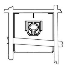
Remove the hood protector, and outline the perimeter of the pedestals with masking tap or the repositionable tape strips supplied to help final installation.
