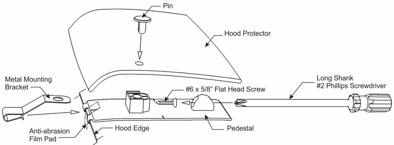
1. Start a #6 x 5/8 flat head screw into each pedestal a few turns. The tip of the screw must not protrude into the hole where the attachment pin will install later. Using a tape measure and grease pencil mark the center of the hood, and positions: **200mm** to the left and right of the center mark. *See Illustration #1.*
