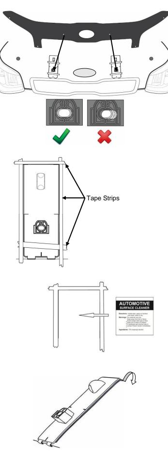
Place the hood deflector on the pedestals to confirm proper positioning. Ensure the holes in the deflector line up with the holes in the pedestals. If necessary, reposition the pedestals so all attachment positions are correct and the deflector is well centered.
