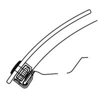
Place a clip body over the anti-abrasion film pad on the edge of the hood.
