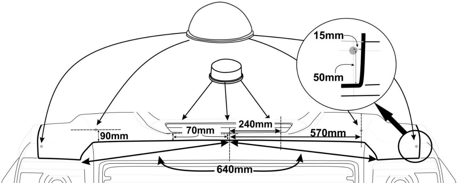
3. Clean the area indicated in the illustration to a point approximately 24" on each side of the center of the hood.
