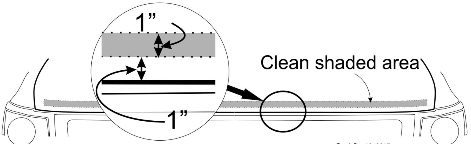
4. Center the "D" gasket laterally on the hood. 48" is provided. It may be necessary to trim the length slightly to fit the contours of the hood.
