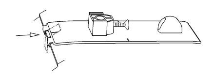
12. Peel and fold the small anti abrasion film pad in half over the hood edge between the fingers on the pedestal.
