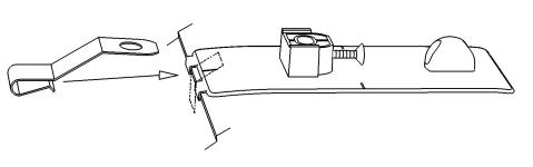
13. Push a metal mounting bracket over the hood edge on top of the anti abrasion pad installed previously. Ensure the bracket is fully engaged over the hood edge and the hole in the bracket is aligned with the hole in the pedestal.
