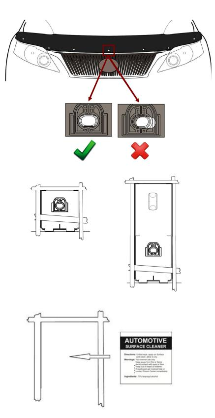
7. Confirm correct positioning of the pedestals, by adjusting the pedestal position on the hood to align with the holes in the hood protector.
