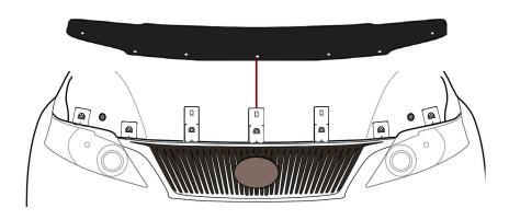
Place the protector temporarily onto the Adhesive pedestals, aligning the holes in the protector with the holes in the pedestals. This step will allow you to confirm the position of the adhesive pedestals.
