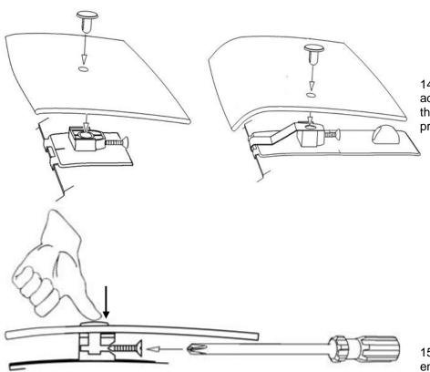
14. Place the hood protector onto the adhesive pedestals mounted on the hood. At the pedestal locations, drop a pin through the protector and into the pedestal.
