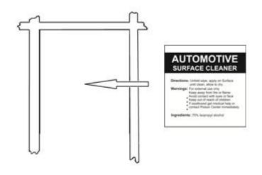
8. Remove the pedestals and thoroughly clean the outlined area with the alcohol wiping pad.
