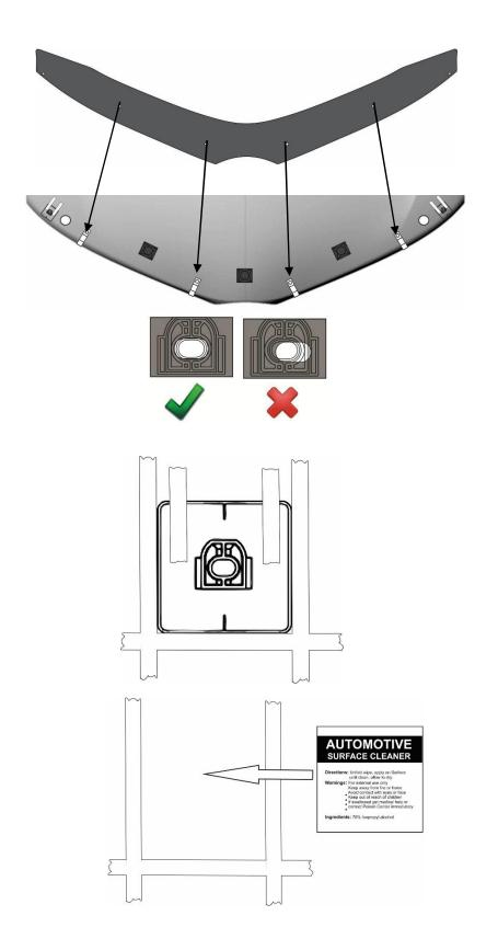
7. Place the protector temporarily onto the metal brackets, aligning the holes in the protector with the holes in the metal brackets. This step will allow you to check the position of the adhesive pedestals and adjust if necessary.
