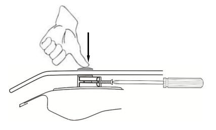
13. Insert a pin through the protector and into each of the two (2) pedestals. Maintain pressure on the head of the pin to ensure the protector is seated against the pedestal and tighten the screw until snug. Do not over-tighten!
