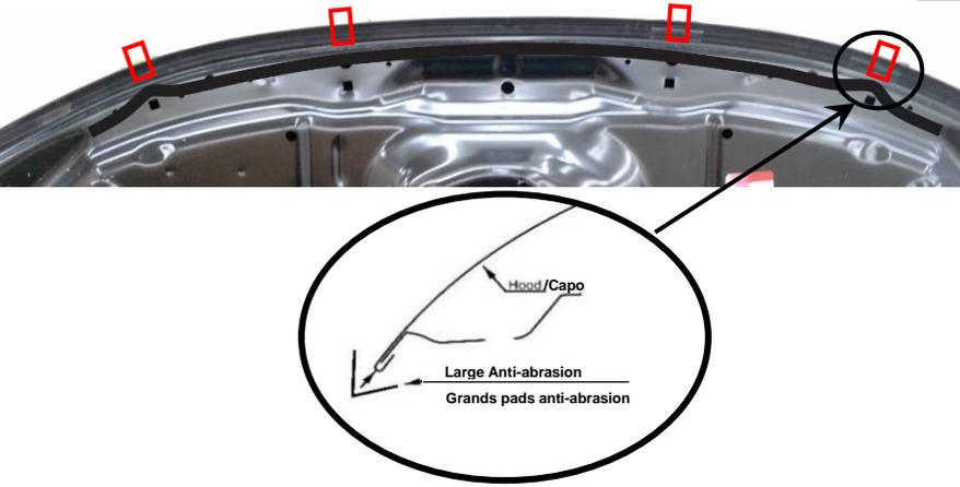
7. Peel protective backing from the large anti-abrasion pads and wrap them around the leading edge of the hood aligned above the expansion plugs installed in step 6. See illustration
