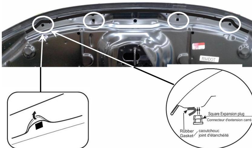
6. Open the hood of the vehicle. Fold back the rubber gasket from the locations shown in the illustration, exposing four (4) square holes. Install one expansion plug into each hole.
