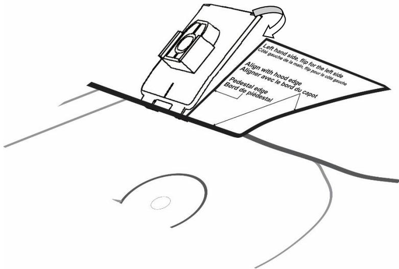
4. Remove the protective backing from the pedestal, align with edge of template and install on the hood surface.
