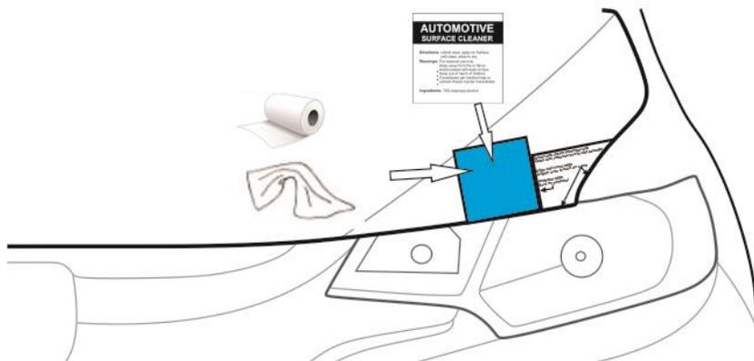
3. Using the automotive surface cleaner, 1st thoroughly wipe the shaded area of hood surface shown in the illustration followed by drying with a soft cloth or paper towel. This will insure all wax, finger prints and oils are removed from the hood surface in the bonding area.
