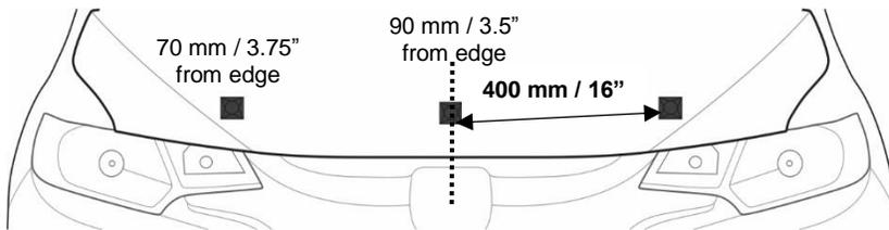
1. Install the three (3) Bumpers as shown. **Attention: the Bumpers must be installed on the hood, not on the protector!!!** If the Bumpers are installed on the protector, they may wear through the paint.
