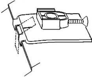
12. Push a type C metal mounting bracket over the hood edge. Align the hole in the bracket with the hole in the pedestal.
