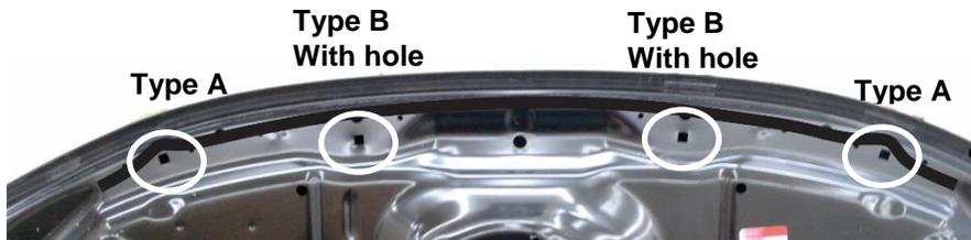
8. Install metal brackets over the hood edge in their corresponding positions making sure to install lower leg of brackets underneath the rubber gasket and aligned with the round hole in the expansion plug. See illustration.
