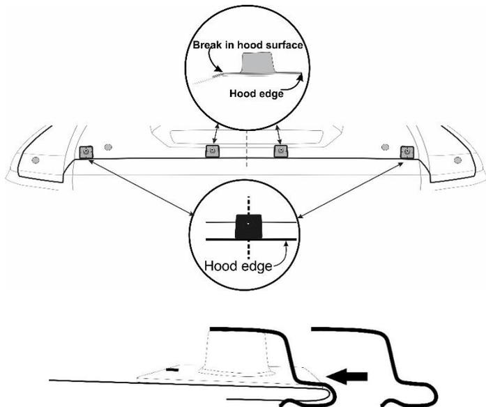
1. Use one of the surface wipes provided and wipe down the area (approximately 15cm (6 in.) from the hood edge) where the hood protector will be installed. Wipe dry with a soft cloth or paper towel. This will remove any wax or grease and will ensure a cleaner surface for the adhesive to bond to.
