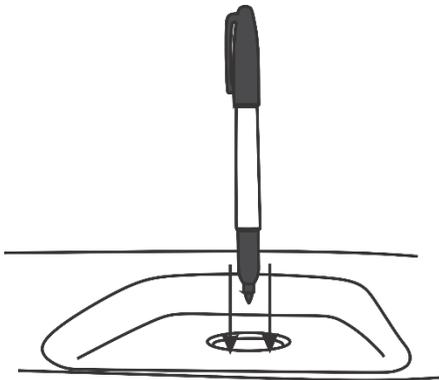
6. With the hood protector in position, locate the two pockets indicated in the illustration. Directly in front of these, at the hood edge, place a small abrasion pad on the underside of the hood. The abrasion pad is oriented with the long edge aligned with the edge of the hood and centered under the pocket.
