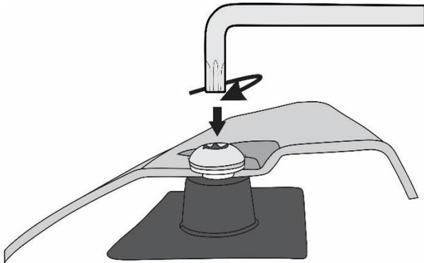
18. Place a Torx head screw through a shoulder washer and into a hole in hood protector. Ensure the shoulder portion of the washer slides into the hole in the hood protector. Loosely thread the screw into the mounting pedestal. See illustration for orientation of the shoulder washer. Repeat for all locations. **Don't forget to install the metal brackets at the two locations from step 6.**
