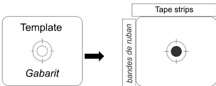
13. Locate the pedestal positioning template and place the template over a dot on the hood. Ensure the template is square to the hood edge. Using two of the repositionable tape strips, outline the template on two adjacent sides. Repeat for all dots. Depending on the application, it may be necessary to cut the tape strips in half to ensure there are enough to outline all locations. **\*\*\*Outline the temporarily installed pedestals as well, then remove them.**
