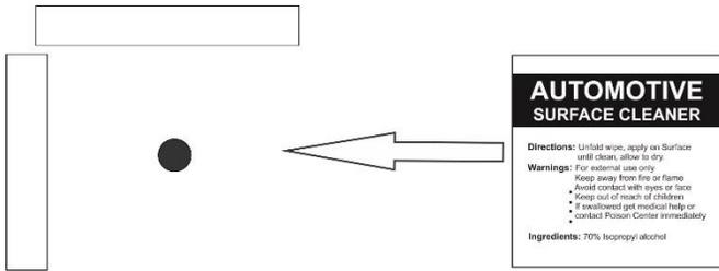
14. Using the automotive surface cleaner provided, clean an area approximately the size of the mounting pedestal at each location. Wipe dry with a clean cloth or paper towel. Take care to not contaminate the hood surface after it has been cleaned. Any surface contaminants will reduce the effectiveness of the adhesive.
