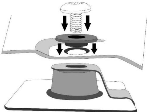
7. Assemble a Torx head screw and shoulder washer as illustrated and thread a screw through the hood protector and into the center pedestal. Check that the hood protector is straight and centered on the hood. Tighten the screw so it's snug but not tight.
