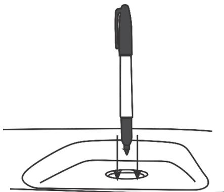
11. Once hood protector is centered, take a felt marker (a fine point Sharpie works best) and insert it into the hole in each of the remaining “pockets” of the hood protector. Keeping the marker perpendicular to the hood surface, mark the hood surface with a dot. **\*\*\*NOTE- IF YOUR HOOD HAS PAINT PROTECTION FILM, A PERMANENT MARKER MAY STAIN THE FILM. USE A DRY-ERASE MARKER OR A GREASE PENCIL.\*\*\***
