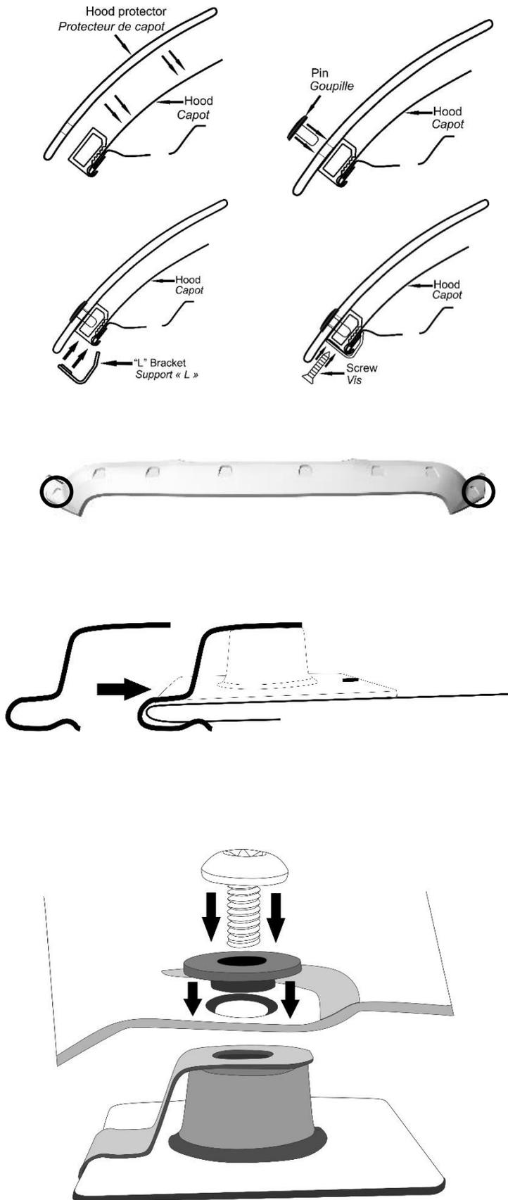
6. With the hood protector in place, assemble the four pieces of the clip body (see illustrations) and loosely attach it to the edge of the hood. Ensure the hood protector is centered and tighten the screws into the clips. Note, the illustrations are generic. This particular hood protector wraps around the edge.
