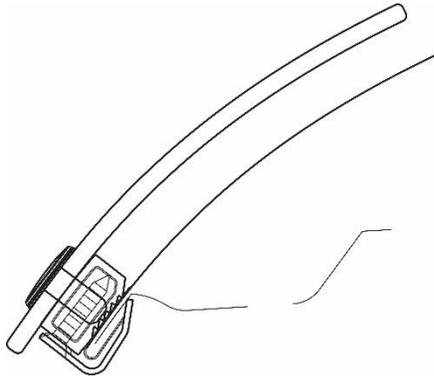
20. Ensure the hood protector is centered on the hood and using a T45 Torx key, tighten the screws into the pedestals. Start in the center position and work outwards. Ensure the shoulder washers are seated properly. Do not overtighten.
