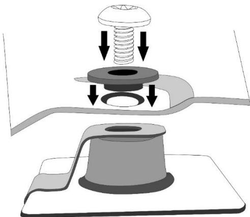
16. Peel the red protective backing off one of the adhesive pedestals. Carefully place it on the hood surface exactly where the tape outline is. **Use care with this step as once the pedestal has been placed on the hood, it will be very difficult to remove.** Repeat for all locations.
