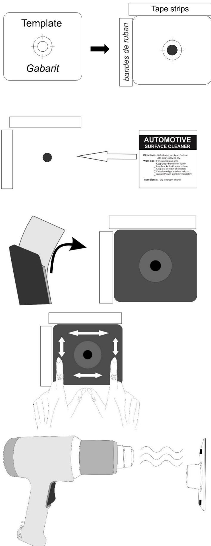
9. Locate the pedestal positioning template and place the template over a dot on the hood. Ensure the template is square to the hood edge. Using two of the repositionable tape strips, outline the template on two adjacent sides. Repeat for all dots. Depending on the application, it may be necessary to cut the tape strips in half to ensure there are enough to outline all locations.
