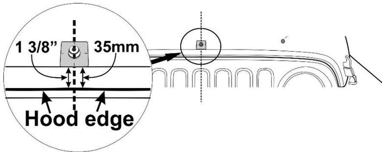
1. Use one of the surface wipes provided and wipe down the area (approximately 15cm from the hood edge) where the hood protector will be installed. Wipe dry with a soft cloth or paper towel. This will remove any wax or grease and will ensure a cleaner surface for the adhesive to bond to.
