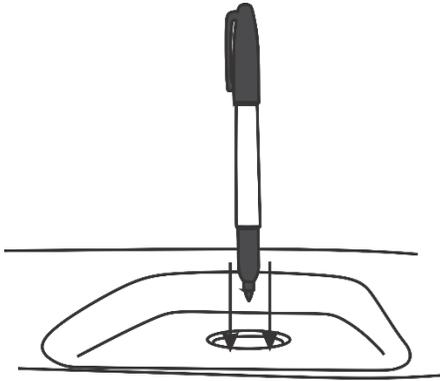
12. Once hood protector is centered, take a felt marker (a fine point Sharpie works best) and insert it into the hole in each of the remaining “pockets” of the hood protector. Keeping the marker perpendicular to the hood surface, mark the hood surface with a dot. **\*\*\*NOTE- IF YOUR HOOD HAS PAINT PROTECTION FILM, A PERMANENT MARKER MAY STAIN THE FILM. USE A DRY-ERASE MARKER OR A GREASE PENCIL.\*\*\***
