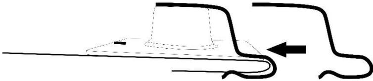
18. Slide metal brackets over the two outer pedestal positions on each side of the hood and place the hood protector on the bumpers and pedestals.
