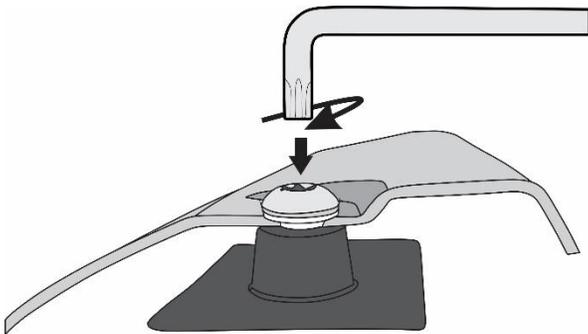
20. Ensure the hood protector is centered on the hood and using a T45 Torx key, tighten the screws into the pedestals. Start in the center position and work outwards. Ensure the shoulder washers are seated properly. Do not overtighten.
