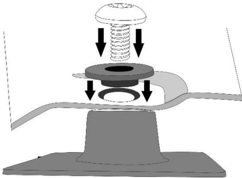
8. Assemble a Torx head screw and shoulder washer as illustrated and thread a screw through the hood protector and into the center pedestal. Check that the hood protector is straight and centered on the hood. Tighten the screw so it's snug but not tight.
