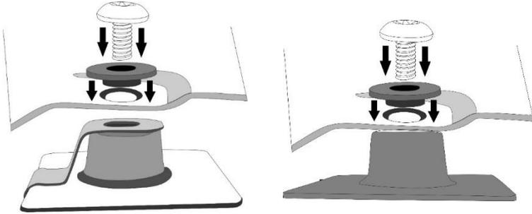
19. Place a Torx head screw through a shoulder washer and into each hole in hood protector. Ensure the shoulder portion of the washer slides into the hole in the hood protector. Loosely thread the screw into the mounting pedestal. See illustration for orientation of the shoulder washer. Repeat for all locations.
