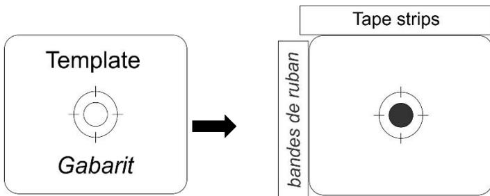
14. Locate the pedestal positioning template and place the template over a dot on the hood. Ensure the template is square to the hood edge. Using two of the repositionable tape strips, outline the template on two adjacent sides. Repeat for all dots. Depending on the application, it may be necessary to cut the tape strips in half to ensure there are enough to outline all locations. **\*\*\*Outline the temporarily installed pedestals as well, then remove them.**
