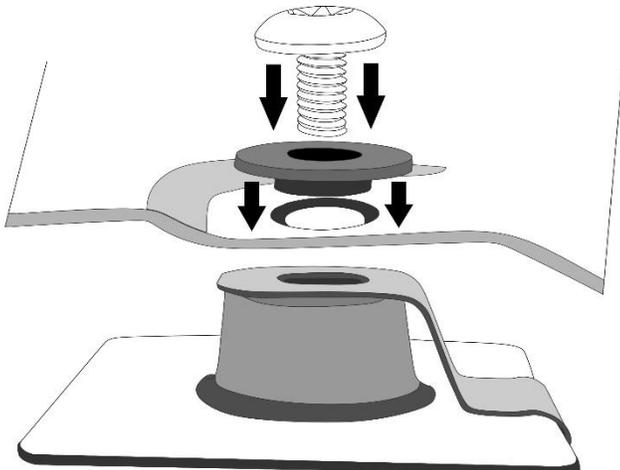
11. As illustrated, assemble a Torx head screw and a shoulder washer and install them in the two positions from Step 10. Only thread the screw in a couple of turns as this is just a temporary step to hold the hood protector in position while other pedestal positions are determined. You may need to adjust the position of the mounting pedestal slightly to align with the hole in the hood protector. Ensure the hood protector is straight and centered on the hood.
