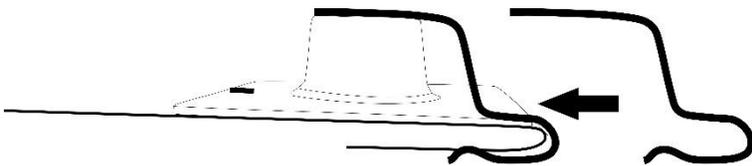
10. Temporarily place a mounting pedestal at the edge of the hood where the abrasion pad is and slide a bracket over each, as illustrated.
